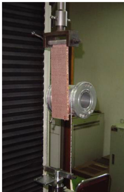
Figure 14. Drum peel test for the composite sandwich plates. This figure is published in color in the online version.
